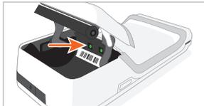
Open the receipt paper door and locate the screws above the serial number (S/N).
