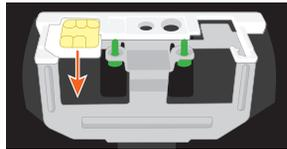
Locate the left tray and remove the current SIM card.
