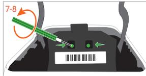
Use the screwdriver to turn the screws counter-clockwise 7-8 times; the screws won't fall out.
