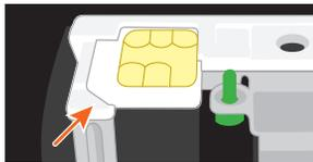
Slide the SIM card into the tray and align it with the angled corner.
